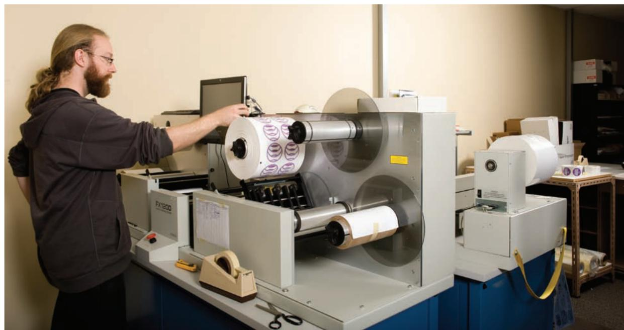
Sticky Business press operator Mike Reid preps the Prima Technology FX1200e Digital Finishing system comprising a die-cutter, laminator, weeder and finisher.
